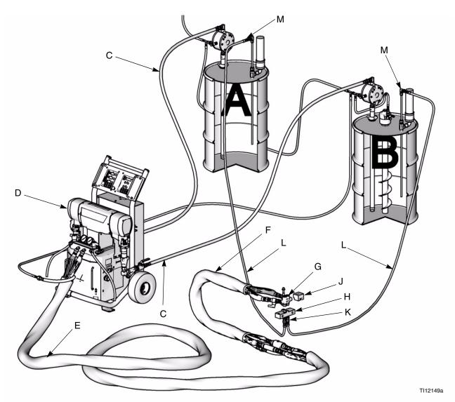
Fig. 1. Circulation System Setup
